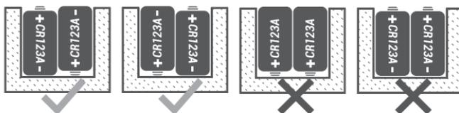
FIGURE 2-2. BATTERY POLARITY
