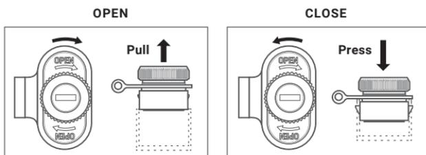
FIGURE 2-1. BATTERY COMPARTMENT
