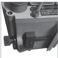
FIGURE 2-3. INTEGRAL RAIL GRABBER ASSEMBLY
