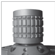
FIGURE 2-14. ILLUMINATOR LENS RECESSED (1 MRAD)
