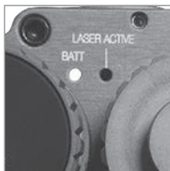
FIGURE 2-16. RED INDICATOR – LOW BATTERY AMBER INDICATOR – EYE SAFE
