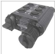
FIGURE 2-8. RMSAL WITH LENS CAPS INSTALLED
